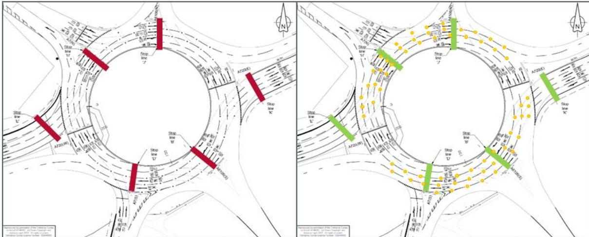
Figure 3: Operation of Road Studs (Signal Phasing Simplified for Clarity)
